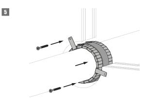
5. Slide the collar into the opening of the wall, in the middle of the wall thickness.
