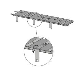
3. Fold the metal plates with pre-drilled holes for 270°.
