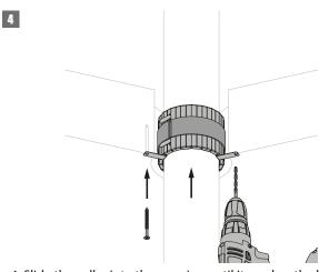
4. Slide the collar into the opening until it reaches the height of the ceiling.
