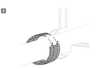
3. Bend the collar and mount it around the pipe. Slide the fastening strips through the corresponding holes. Fold back the strips.
