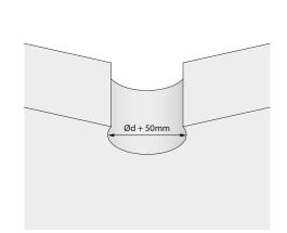
1. Provide an installation opening of Ød + 50 mm.
