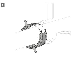
4. Bend the collar and mount it around the pipe. Slide the fastening strips through the corresponding holes. Fold back the strips.
