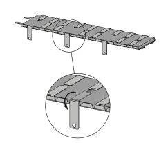
2. Fold the metal plates with pre-drilled holes for 270°.
