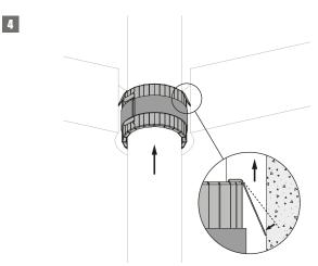
4. Slide the collar into the opening until it reaches the height of the ceiling.
