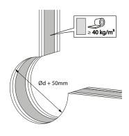
2. Provide an installation opening of minimum  $\emptyset$ d + 27 mm and maximum  $\emptyset$ d + 50 mm for pipe diameters 32-75,  $\emptyset$ d + 36 mm and  $\emptyset$ d + 50 mm for pipe diameters 80-110,  $\emptyset$ d + 40 mm and  $\emptyset$ d + 50 mm for pipe diameters 125-160.
