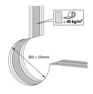
2. Provide an installation opening of  $\emptyset d + 50$  mm.
