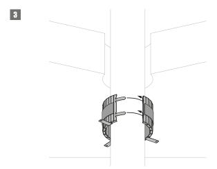
3. Bend the collar and mount it around the pipe. Slide the fastening strips through the corresponding holes. Fold back the strips.
